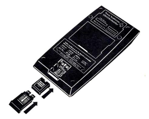
Don't touch the contacts inside the module compartment as damage can result.
