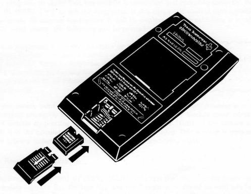
Don't touch the contacts inside the module compartment as damage can result.
