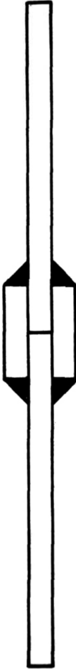
A. COVER PLATE TYPE JOINTS
