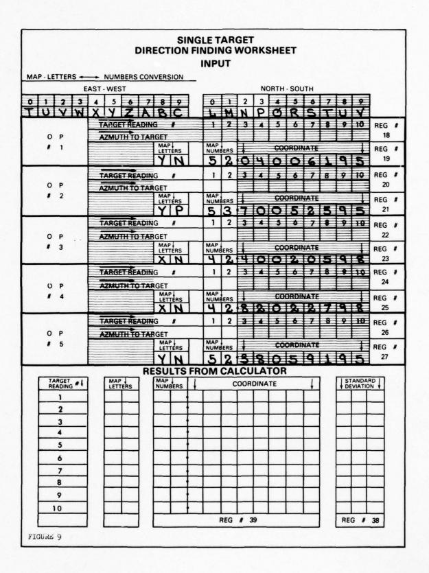
F. Post the OP azimuths. See Figure 10. Gather the azimuths from the OP's and enter them in the "AZIMUTH TO TARGET" row in the next available "TARGET READING #" column (e.g. OP # 1 azimuth is 330 degrees, enter 330 in the appropriate block).
