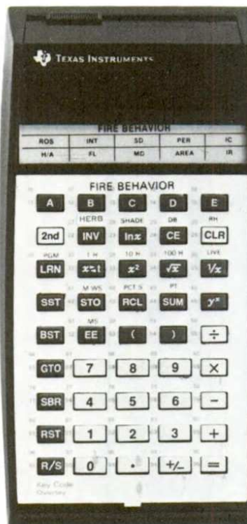
Figure 25.--Modify the fire behavior keyboard overlay by placing the label HERB above the INV key on the calculator.
