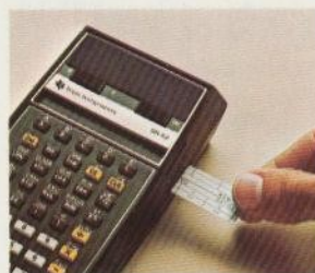
Insert the prerecorded magnetic card. (A side). Remove card. Send it through again. (B side).
