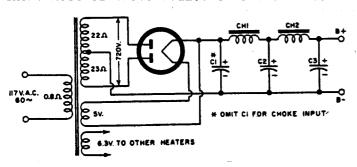
on the left. You might say:"In these days of transistors and ICs, what is that old mastodont good for?" Note the 720 volts high voltage winding. Note also the 110 volts primary winding. Divide one by the other and you get a ratio of roughly 6.5 to 1. Now if you apply 110 volts where normally the 720 would go, you would measure on the other side (where normally the 110 would be connected) about 17 volts.
