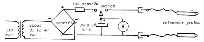
insides. While the dendrite proved to be conductive, it definitely was identified as the villain who shorted my battery. A simple application of about 50 volts evaporated said dendrite. Thusly, the Zapper was born.
