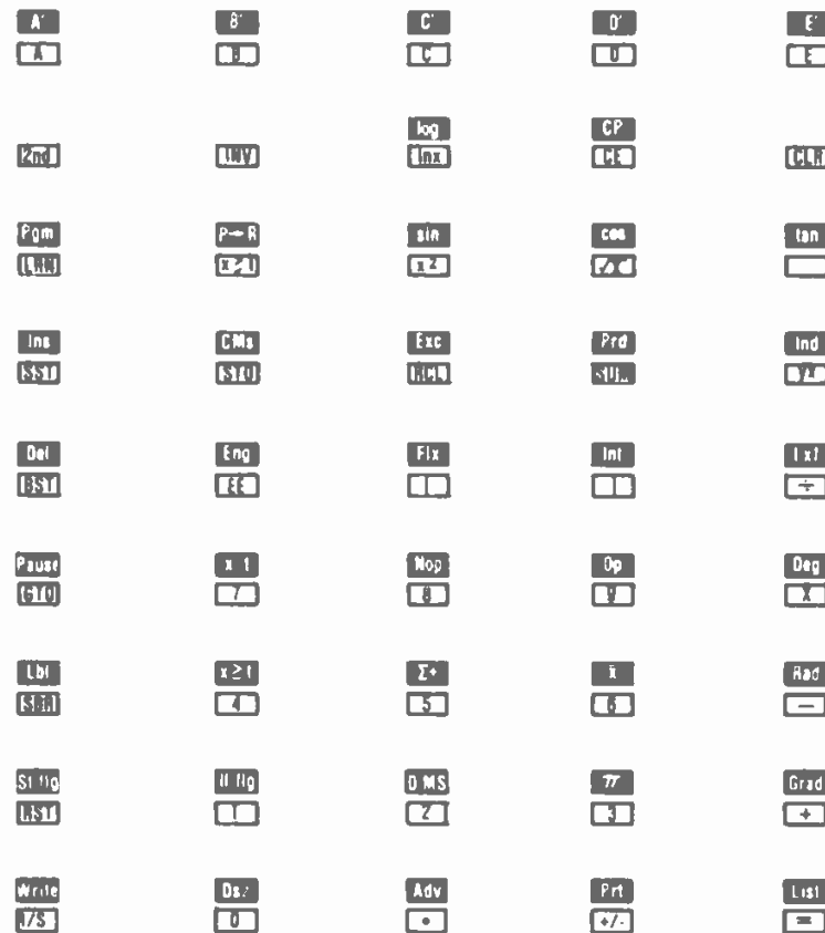
Fig. 4—Keyboard diagram for TI-58. There are two functions for most keys. The basic functions are shown as white keys with black lettering. The second functions, black rectangles with white lettering, are obtained by depressing the (2nd) key and then the key beneath the desired function.
