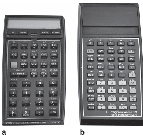
Figure 1. The HP-41CV and TI-59 programmable calculators. Due to its alphanumeric capabilities, (a) the HP-41CV had fewer keys but more functions than (b) the TI-59. The TI-59’s advantages included numerical precision and simpler access to synthetic functions.
