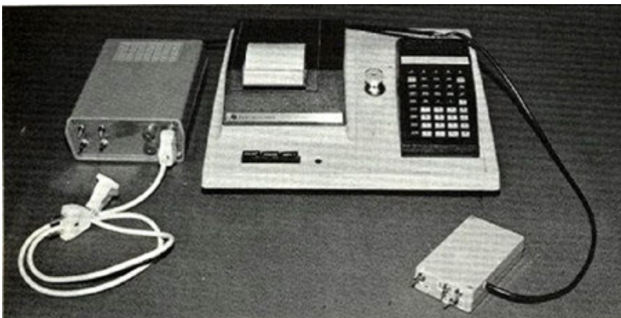
General view of the system with pocket calculator, printer and switching interface with connecting cables.
