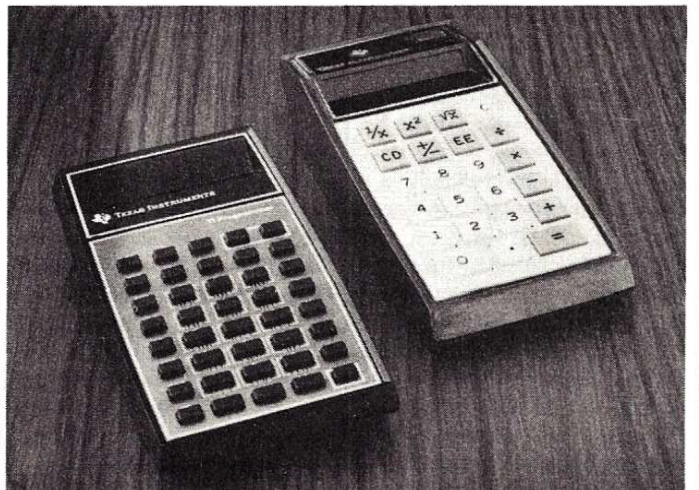
Photo 2. Comparison of Programmer and SR-10 shows the latter's more convenient operating stance.
