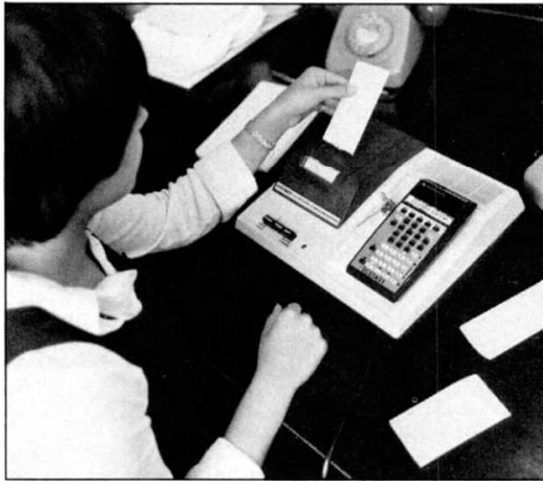
The ECS Ecstasy machine, incorporating a Texas Instruments TI-58 programmable calculator with a 'Custom CROM' program module.
